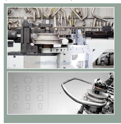
With to high-strength materials or high -strength stainless steel, our benders prevent the formation of badly looking marks due to slippage at the end of the deflection, and premature wear of the tooling.
